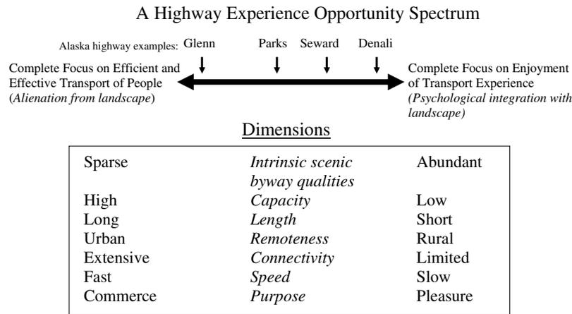
Fig. 4. A proposed highway opportunity spectrum based on highway attributes and proposed placement of selected Alaska highways.
